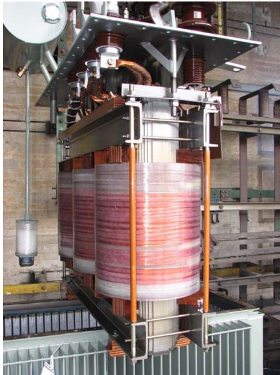
Fig. 5 Side view (phase A) of active part after all tests
