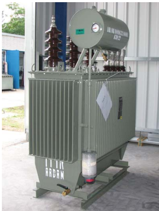
Fig. 2 Tested transformer (LV terminal side) after short-circuit test
