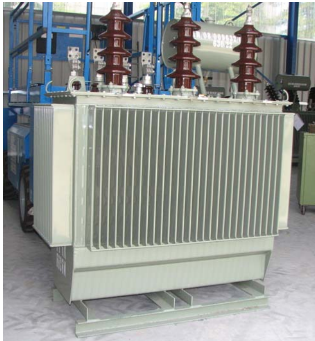
Fig. 1 Tested transformer (HV terminal side) after short-circuit test
